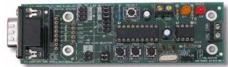
Fig.3 E-blocks CAN controller and line driver
